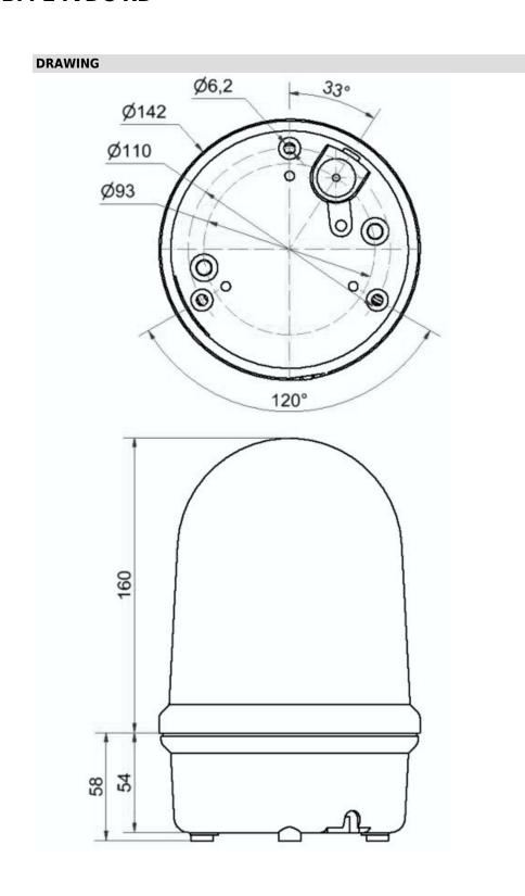
For additional installation and mounting information, refer to the appropriate user guide at www.werma.com. This printed copy is for information only and is subject to alteration.
